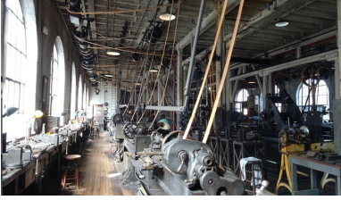
Belt Drive machines powered by remote steam engine
