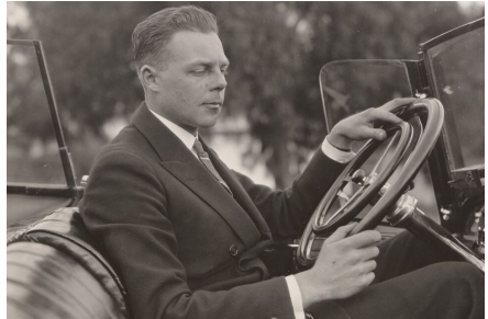
Doble Driving: Abner Doble at the helm. The inner wheel controls the vehicle’s speed. (Doble Steam Motors Corporation Photograph Collection)
